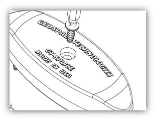
\*NOTE: THE TOP IS ROTATED 180 DEGREES FOR SHIPPING PURPOSES AND WILL NOT CLOSE IN THIS POSITION.
